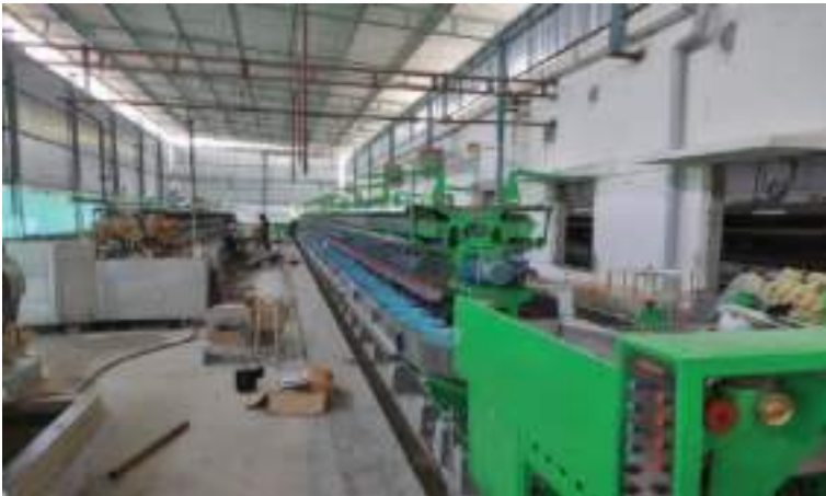
Automatic Dupion Silk Reeling Machine Unit, Udumalpet
